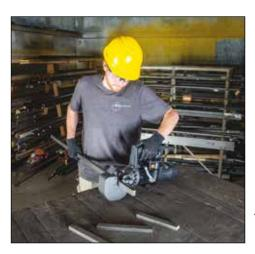
Cutting flat bar is fast and easy with EFBE-Series Electric Flat Cutters.
