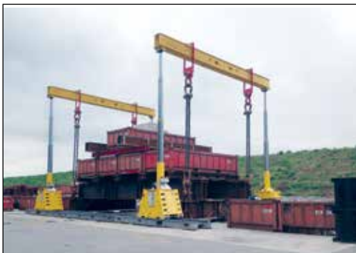
◀ SL-400 Gantry during load testing.
